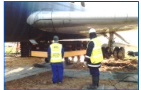
The Trident aircraft being lowered onto cribbing and Transporter using aircraft recovery airbags.
