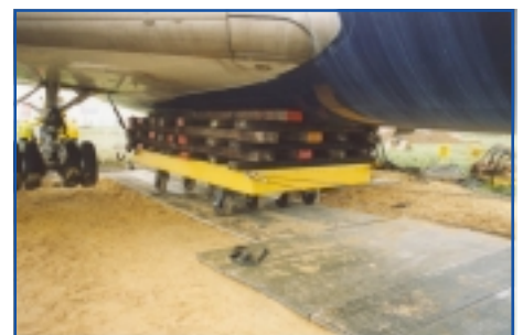
The full weight of aircraft is supported on the Transporter. Trakcess panels have been laid on soft ground to aid the recovery.
