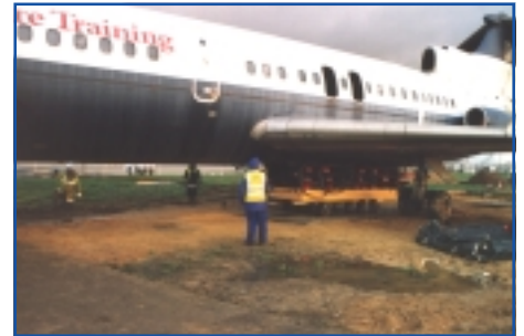
The AMS Transporter system was used at Heathrow Airport under a Trident Aircraft during a recent recovery exercise.
