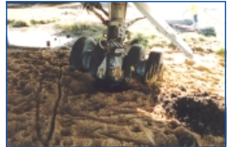
The landing gear on the Trident was seized solid, therefore the Transporter had to be used to move the aircraft to its new resting place.
