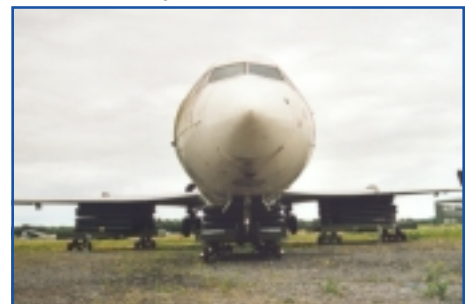
Multi Transporter system. 3 transporters used for full landing gear failure.
