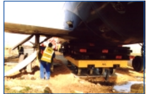
This photo shows the versatility of the Transporter, even on soft ground used with AMS Trakcess panels, a recovery can be completed.
