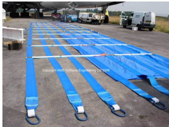
View of A380 fuselage sling - Length 21m - 8 slings pitched to suit A380 frames
