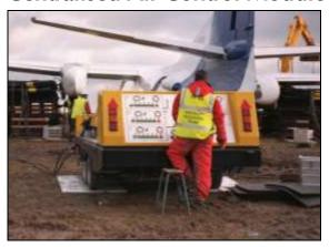
The Centralised Air Control Module [CACM], is unique to AMS, and has been developed as a rapid deployment air inflation system for aircraft lifting bags. The central control panel allows the operator independently inflate up to 75 air bags at 5 points around the aircraft.
