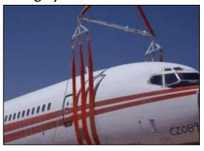
AMS have developed a fuselage lifting system that is universal for the majority of aircraft which are operational in today's industry.
