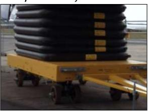
Should the aircraft experience a landing failure on the runway or other hard standing, the AMS transporter system enables the aircraft to be removed from the incident site quickly and effectively, minimising the down time often experience when waiting for third party assistance.
