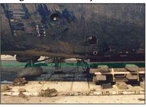
In the event of a landing failure on soft ground, the AMS sledge system enables the aircraft to be removed from the incident site, without the need for specialist transportation systems.
