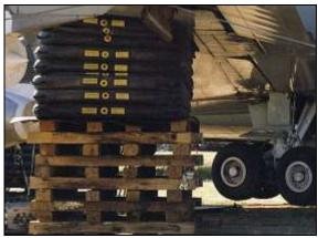
Air Bags are available in various capacities and can be manufactured as either single element, module or multi stack configurations.
