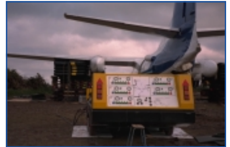
The Centralised Air Control Module positioned at the rear of the Aircraft.
