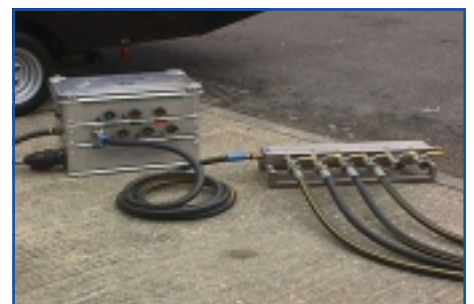
Remote Control Console and Air Distributor connected by air supply hoses.
