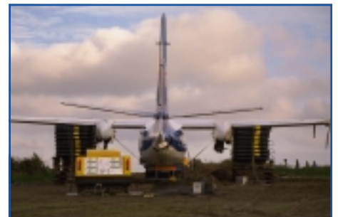
Aircraft raised and ready for lowering onto a flatbed Trailer.
