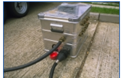
Remote Control Console with Air Supply Hose and Remote Control Manifold hoses attached.
