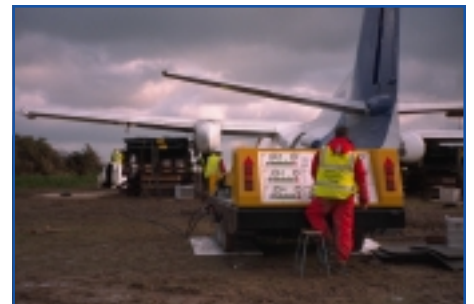
Inflation of the Airbags in progress. The operator has good visibility of all lifting points.
