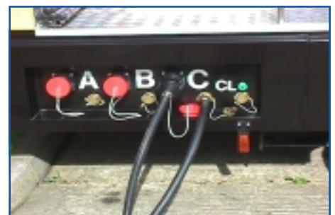
Outlet points on the side of the Centralised Air Control Module. Air Supply Hose and Remote Control Manifold hoses are connected.
